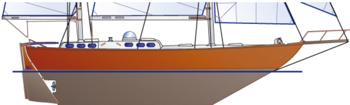
Exemple of rudder separated from the keel (here with a classique keel, ie with garboard strake)
